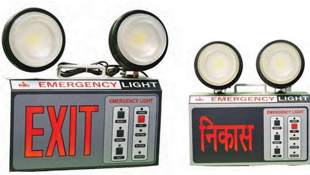
Twin spot emergency luminaries with 3 switches, each lamp spot can be switched on/off through tactile switch. Each lamp has 10W LEDS to supply high luminance.
