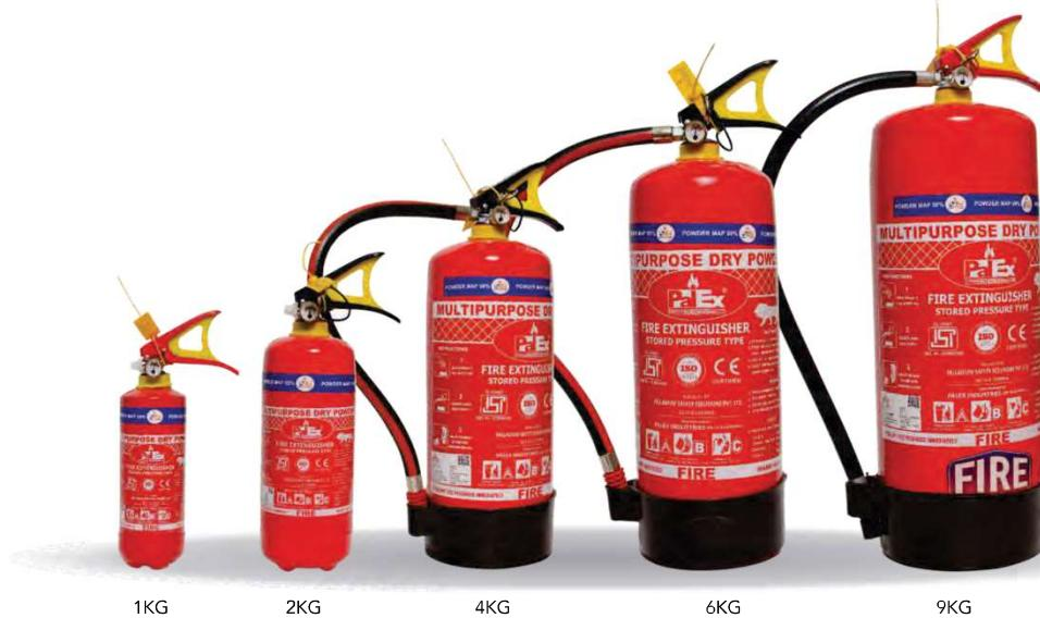
ABC fire extinguishers are often the ideal choice because they can put out many different types of fires. They use a dry chemical known as monoammonium phosphate that can quickly put out the fire. It is a pale-yellow powder that is used to extinguish three classes of fire. ABC fire extinguishers are considered "multi-purpose" extinguishers which can be used on Class A, B, C fires as well Electric Fire.
