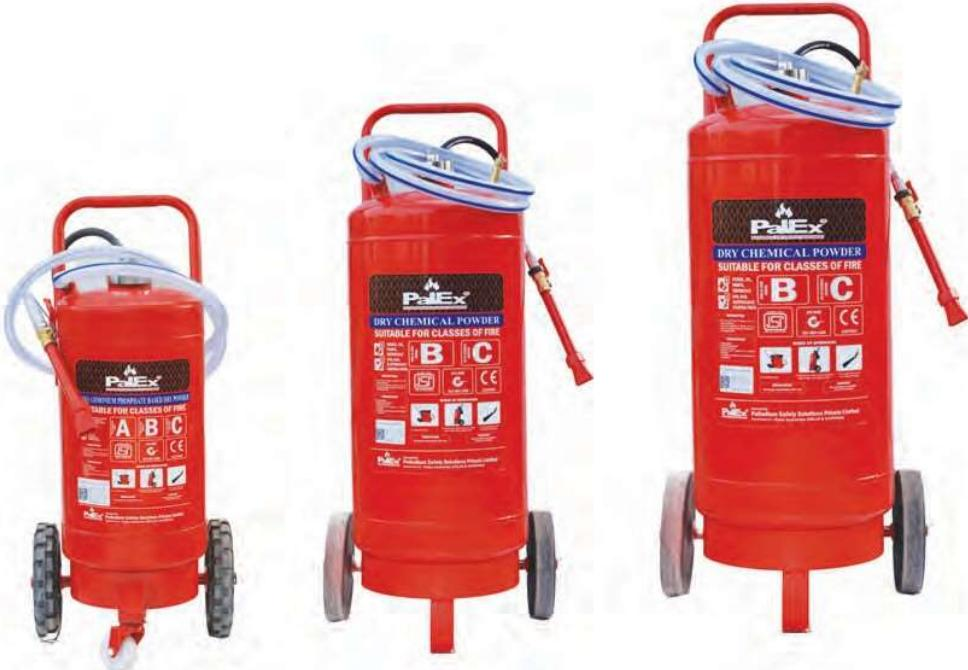
ABC fire extinguishers are often the ideal choice because they can put out many different types of fires. They use a dry chemical known as monoammonium phosphate that can quickly put out the fire. It is a pale-yellow powder that is used to extinguish three classes of fire. ABC fire extinguishers are considered "multi-purpose" extinguishers which can be used on Class A, B, C fires as well Electric Fire.
