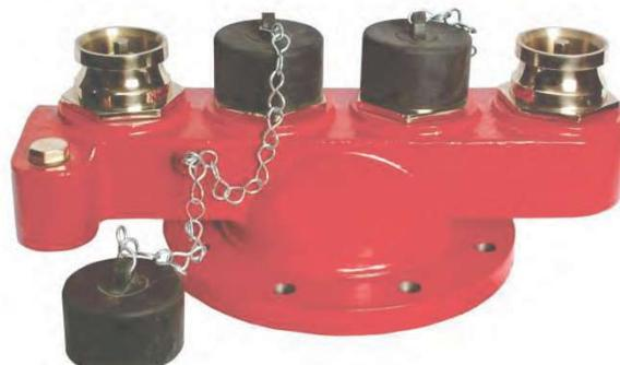
Fire Brigade Inlet allows Fire Tenders to pump in water into the Dry Riser/ Wet Riser/ Sprinkler system piping using external water sources such as hydrants. Fire Brigade Inlet is fitted with required number of standard Male Instantaneous inlets to feed the Riser pipe.
